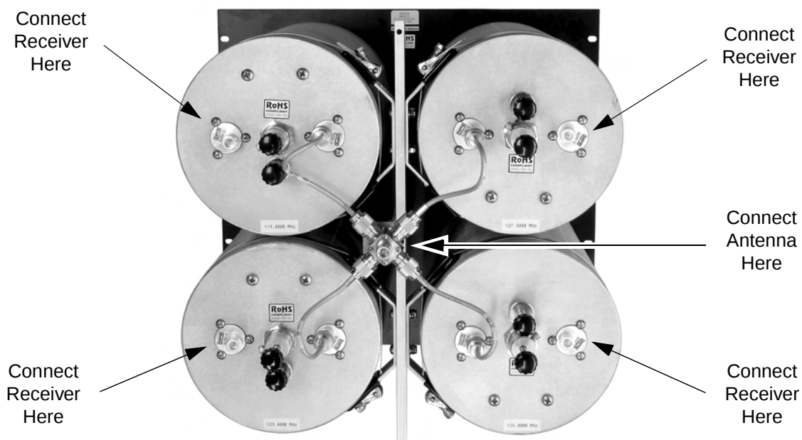
Figure 2: Interconnecting the four channel system.
